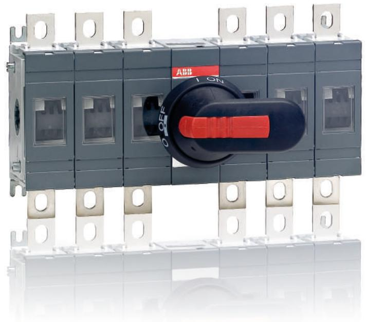
The calculations have now given us a picture of the requirements for the switch-disconnector, and the decision can be made. For example, the ABB's OT250E33 is rated at a  $U_g$  of 1000 V and an  $I_g$  of 200 A, DC-21 B, and would thusly be an ideal choice.
